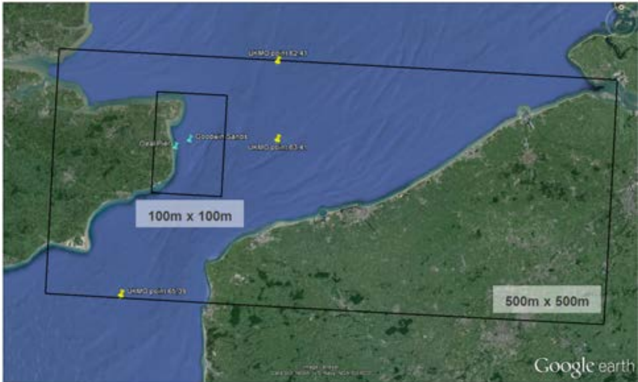
Figure 3.1: SWAN wave model extent and grids, UKMO European Waters model grid points (yellow pins) and wave measurement locations (blue pins)
