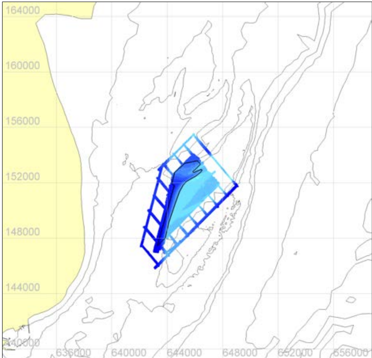
Figure 2.1: Spatial extent of the 2015 bathymetric survey of the Goodwin Sands, with proposed dredge area indicated by the black polygon
