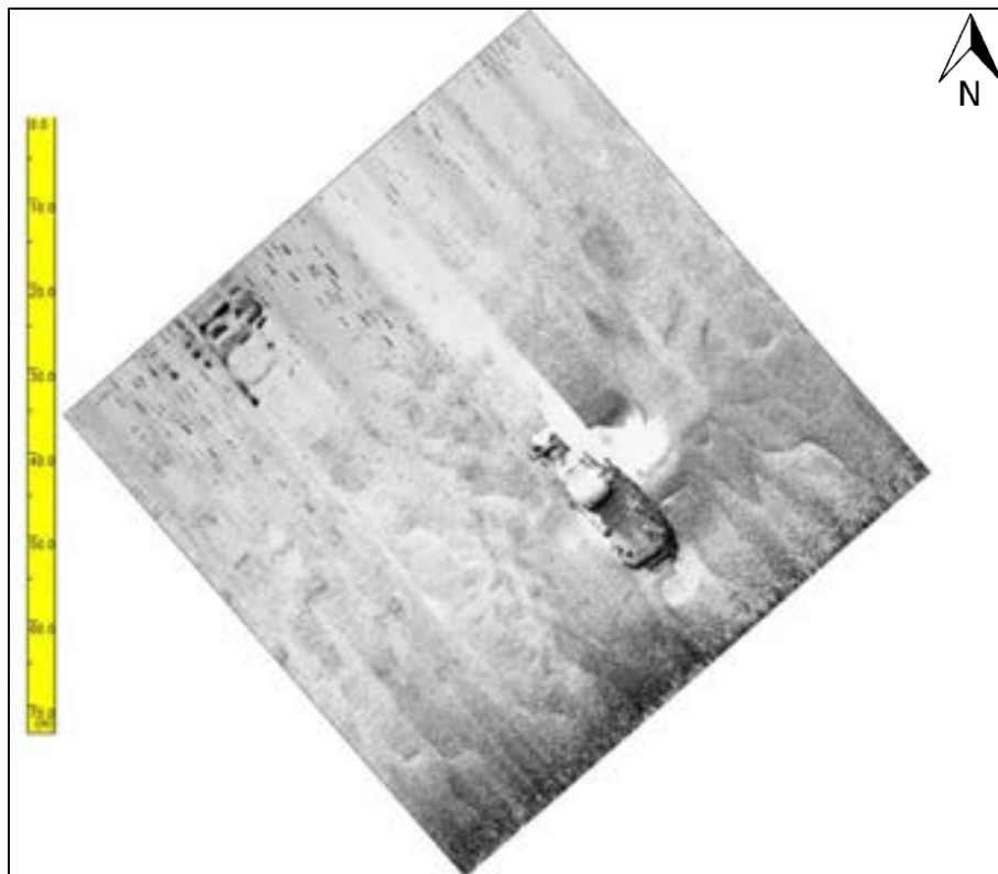
FIGURE 14: SSS IMAGE – REMNANTS OF THE STERN SECTION OF THE ‘SS NORTHEASTERN VICTORY’ WRECK
